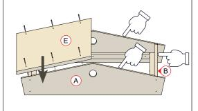
Place Item **F** (x2) onto Item **E** (x2) and secure around **edge** with 14 short galvanised nails.
